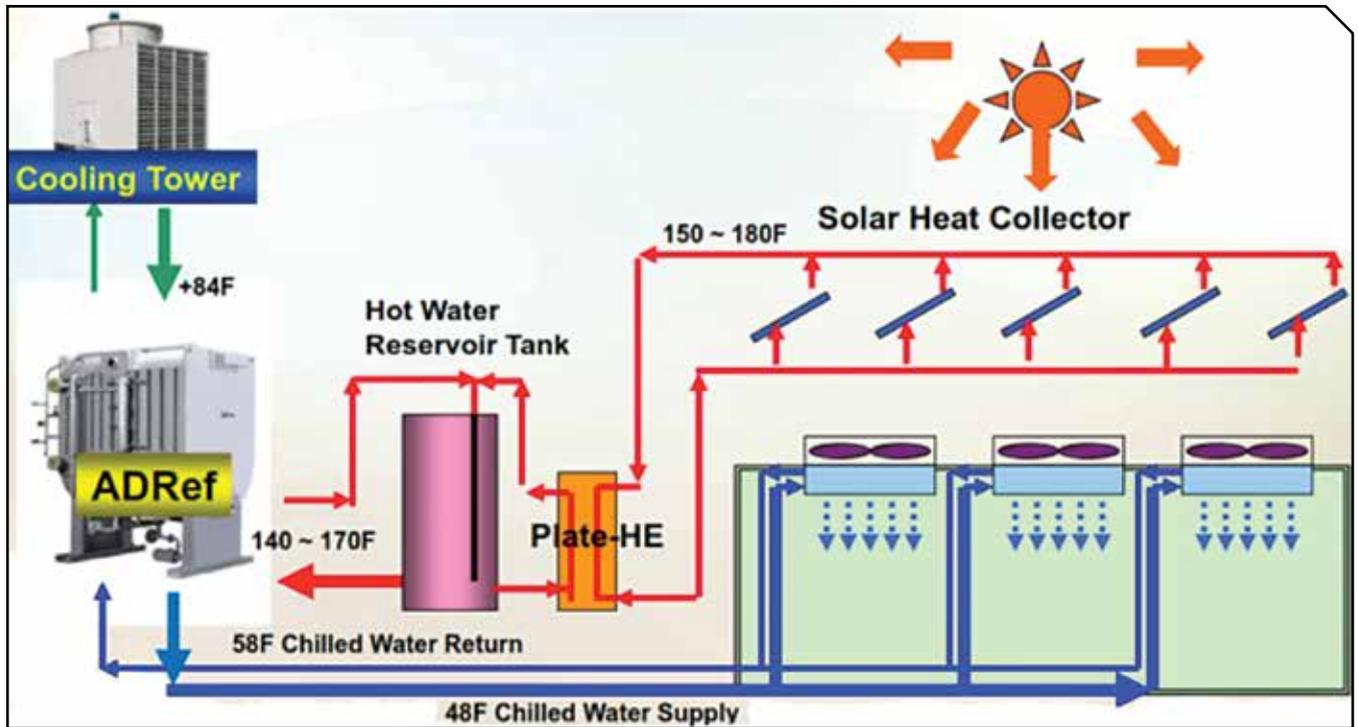
**FIGURE 1.** Low-temperature adsorption waste heat chiller (Source: Mayekawa).
